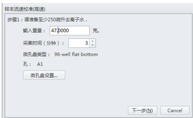
Sample flow rate calibration (High speed) dialog box. It contains the following fields and buttons:
