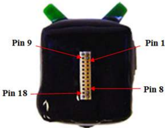
Figure 7: .025" Omnetics Female TBSI P/N: A9094 Mating Male Electrode Connector TBSI P/N: A8784
