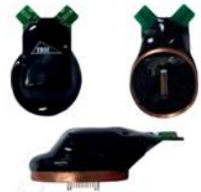
Figure 26: Inductive Power Headstage
