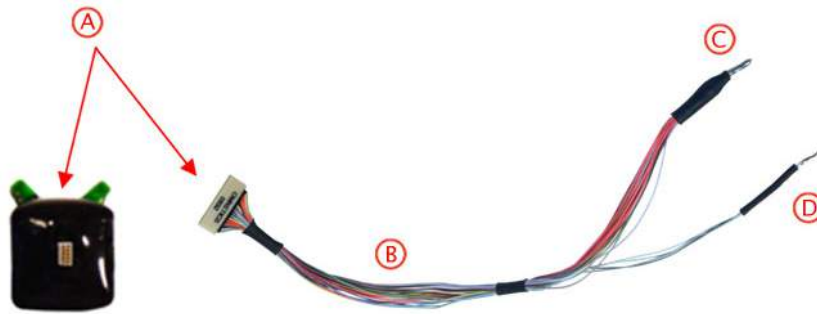
Figure 16: Headstage and Signal Transmission Test Cable
